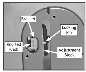
**Figure 38.** Knurled knob used to secure the spreader.
